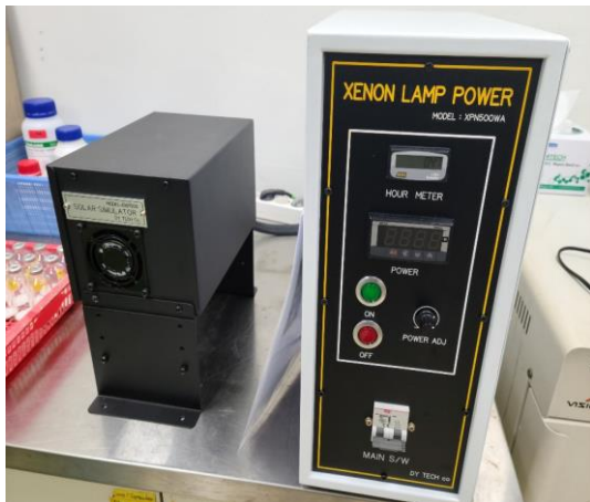
Photoreactor for photodegradation
